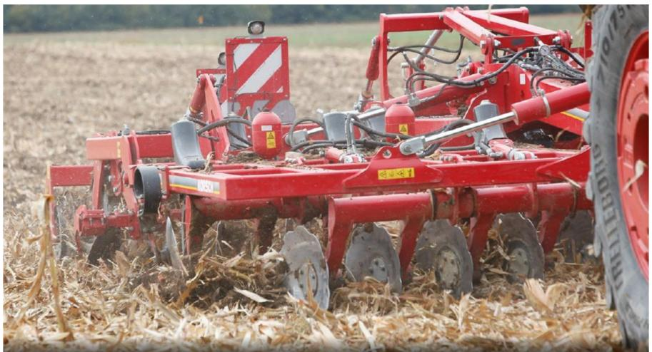
• Fuel miser: The Horsch Tiger MT four-in-one cultivator reduces the number of passes over a paddock, leading to fuel savings of up to 25 litres per hectare.
